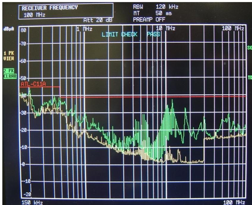
**Figure 11. Measured 200V Vout channel at STBY regime.** The yellow spectrum – HPS1 power supply ch1 is still switched OFF, all cooling ventilators are ON. The green curve –HPS1 is already ON in standby mode. We can already distinguish the 200kHz switching frequency peak of the DC/DC converter, as well as increasing spectrum at 7-30MHz. It is still below the ATLAS emission limits.
