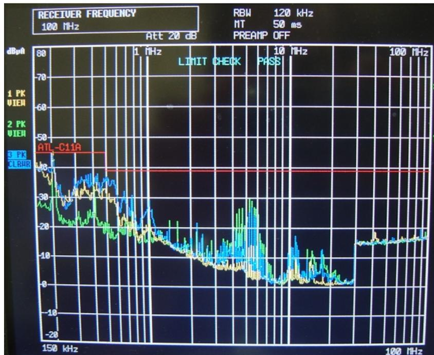
**Figure 10. Initial measurements.** Comparison of conducted noise measurements for three output channels, all cooling fans for dummy loads and HPS1 are ON, HPS1 power supply is still switched OFF. The Yellow curve - ch1 - as on previous Figure 9, Green curve - ch2, Blue curve presents ch3 cable spectrum, respectively. We can see spectral differences from channel to channel already at low frequencies 150kHz – 1MHz.
