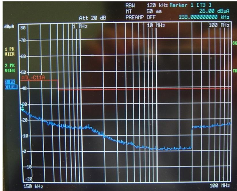
**Figure 7. Initial measurements.** Background conducted noise with the current probe on the air. All cooling ventilators for dummy loads and HPS1 are running; HPS1 itself is OFF. The observed increase at 30MHz is caused by wider frequency step and wider resolution BW of the spectrum analyzer, see Table 1. The red line is the ATLAS conducted emission limit, see also Table 2.
