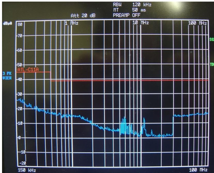
**Figure 8. Initial measurements.** Background noise of Vout channel 1 cable (1m long), all cooling ventilators and HPS1 power supply are OFF.
