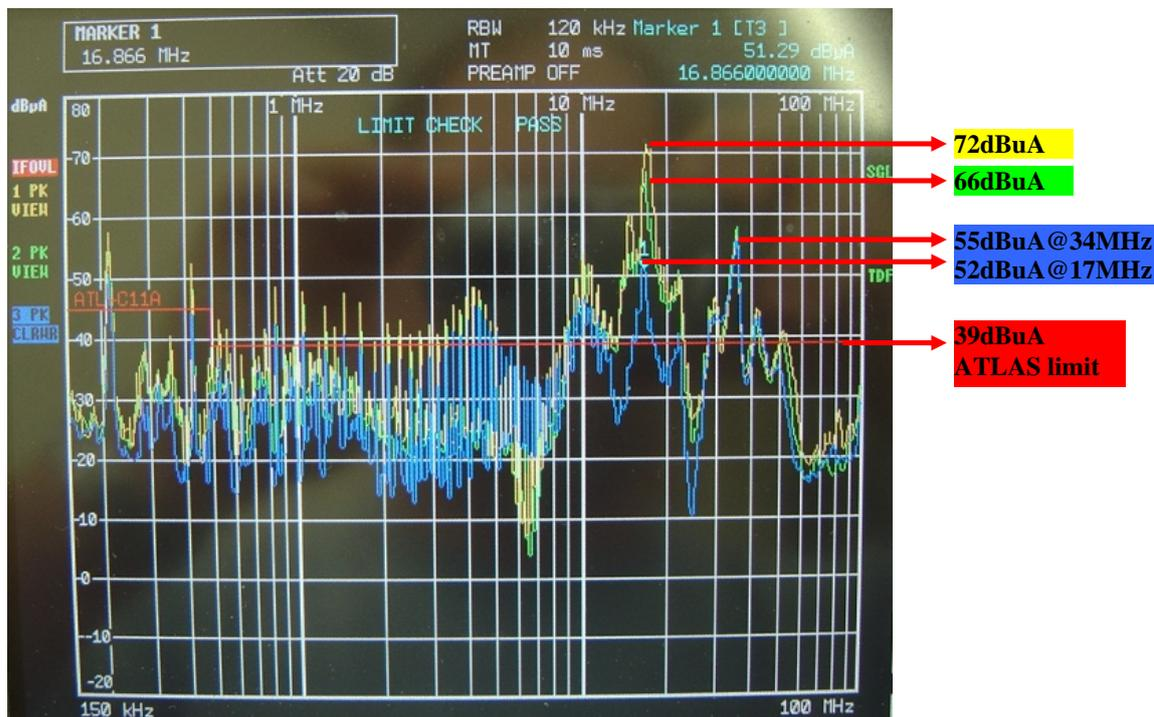
**Figure 15. Comparative measurements of 17MHz peak suppression:** without ferrites (yellow curve, the same as on Figure 13), with one ferrite (green curve), and with two ferrites mounted on 200V cable (blue spectrum). The HPS1 Vout conducted emission spectrum; ch1 is ON and loaded by resistive equivalent load.
