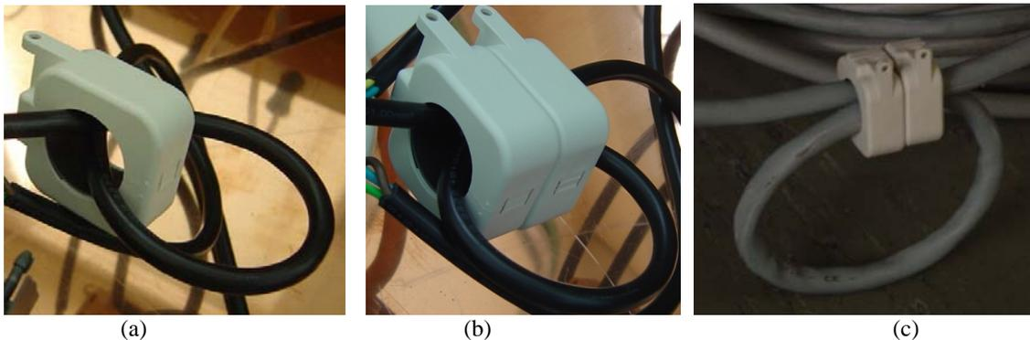
**Figure 14.** Common mode suppression ferrites with appropriate diameter that enables 2times through ferrite configuration. Photos with one (a) or two (b) mounted ferrites on 200VDC Vout cable. Photo (c) demonstrates the original 200V cable with 2 ferrites setup proposed for the ATLAS USA15 tunnel.
