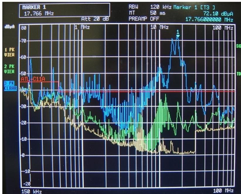
**Figure 12.** HPS1 ch1 is ON and loaded by an equivalent resistive load (blue curve). The power delivered to the dummy load is 737W. The yellow and green spectra are the same as from Figure 11. We see very high and disturbing peak at 17.7MHz (72.1 dBuA; compare to the ATLAS limit of 39dBuA) as well as increased spectrum from 6 to 22MHz.
