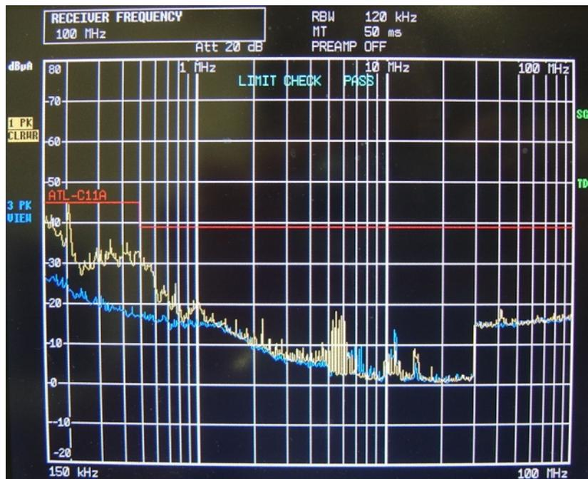
**Figure 9. Initial measurements.** Blue curve – previous conducted noise measurements of one meter Vout cable from Figure 8, Yellow curve – additional conducted noise created when all cooling ventilators are turned ON; the HPS1 power supply is still switched OFF.
