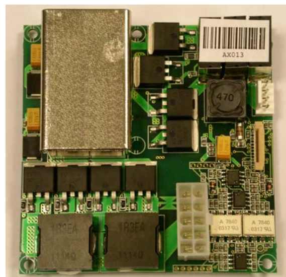
Figure 4: TileCal DC/DC converter 80x80mm.
