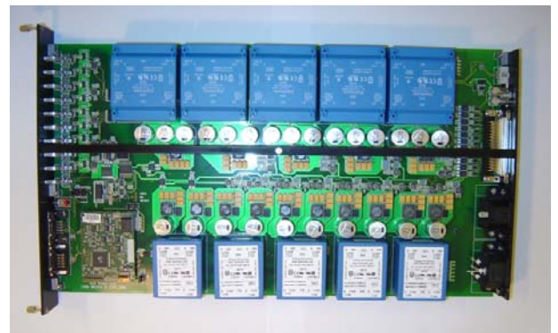
Figure 7: LVPS AUX board photo.
