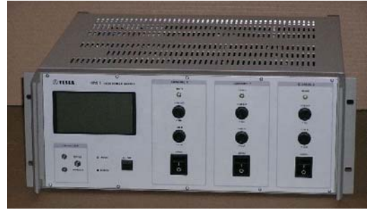
Figure 6: HPS1 200V DC power supply photo.
