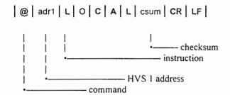
Remote: switches the HVS I over into the remote mode of operation
