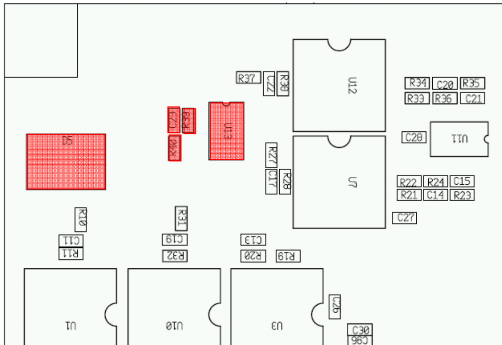
Fig.6. Unsoldered components from bottom side ELMB_MBv6.5 related to point 3-e.
